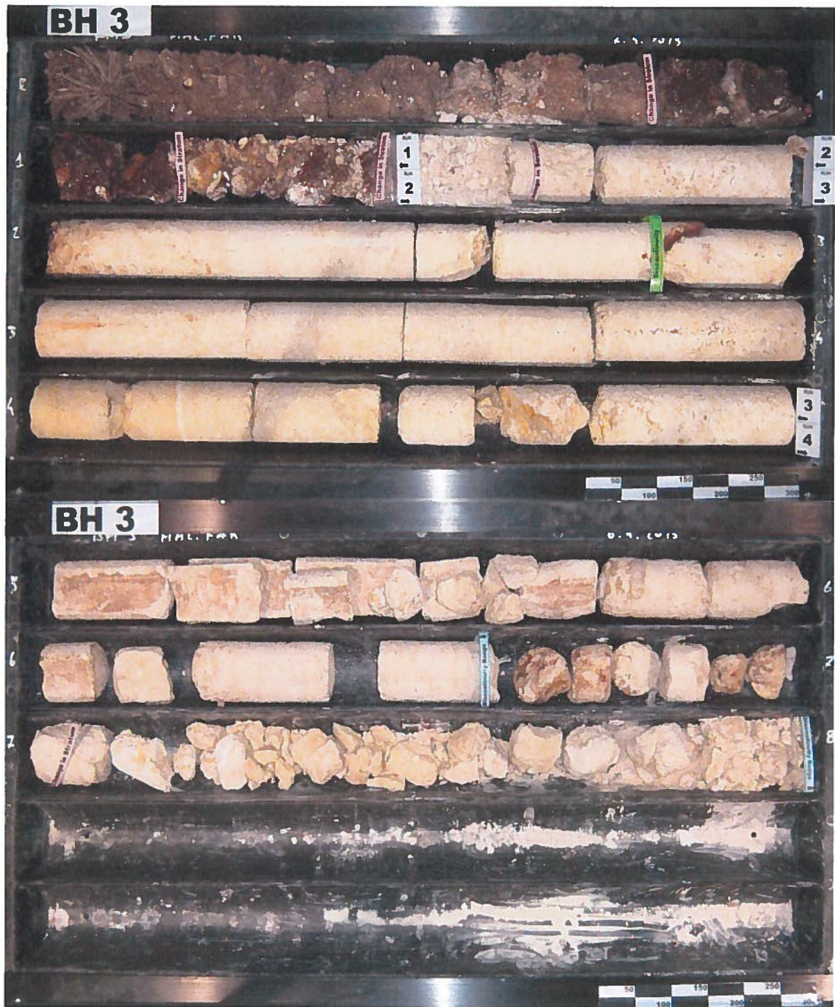
Figure 13 - Retrieved core from borehole 3
