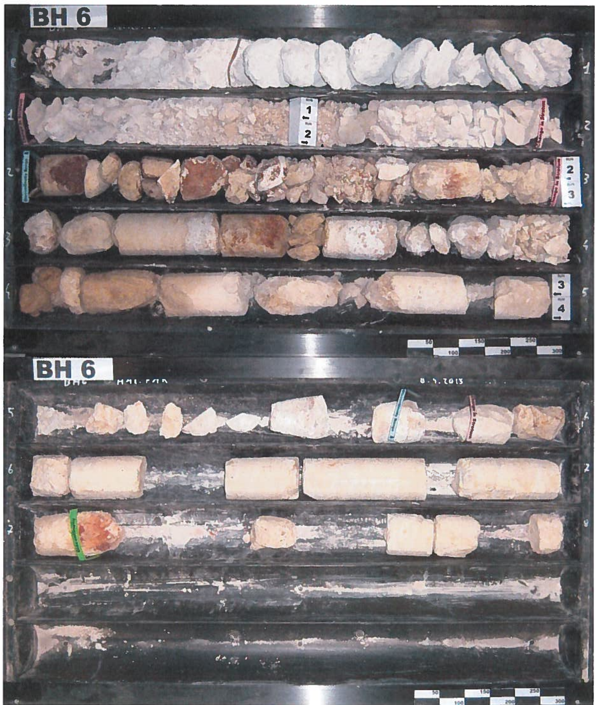
Figure 16 - Retrieved core from borehole 6
