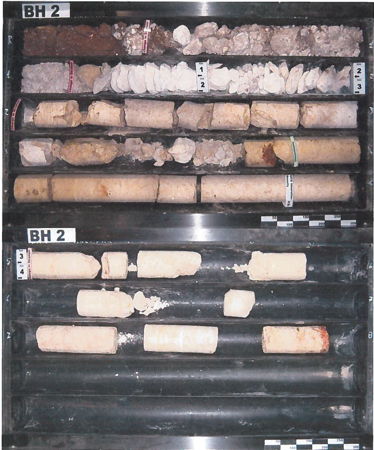
Figure 12 - Retrieved core from borehole 2
