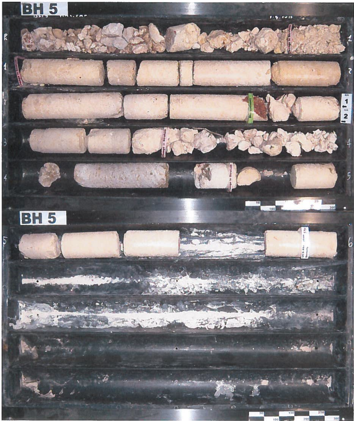
Figure 15 - Retrieved core from borehole 5
