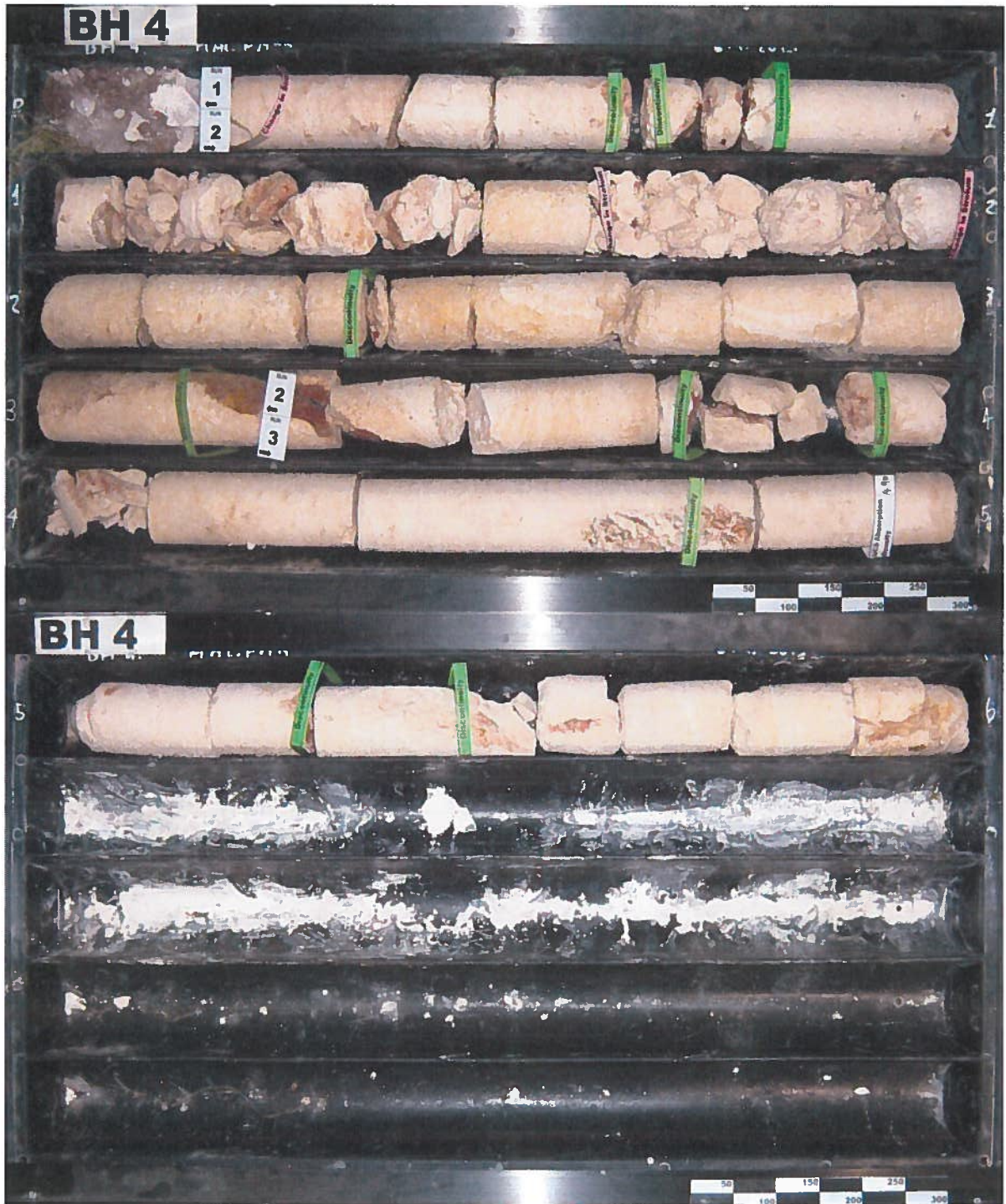
Figure 14 - Retrieved core from borehole 4
